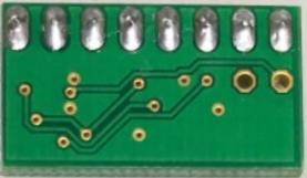
8-pin pin-header assembled to the top-side of the USB-module
