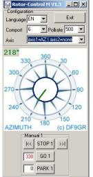
Configure the Axis to <axis1=AZ | axis2=none>.
