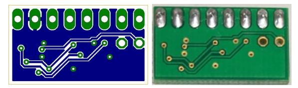
8-pin-header assembled and soldered to top-side of the USB-module
